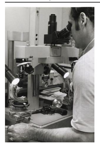
An electronic microscope takes photos of the pistol barrel. Items are microscopically tested to show indentations and markings found on the weapon and on the bullet, NYC
