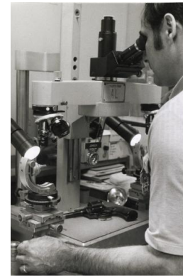
Title: An electronic microscope takes photos of the pistol barrel. Items are microscopically tested to show indentations and markings found on the weapon and on the bullet, NYC Date: 1975 Primary Maker: Leonard Freed Medium: Vintage gelatin silver print
